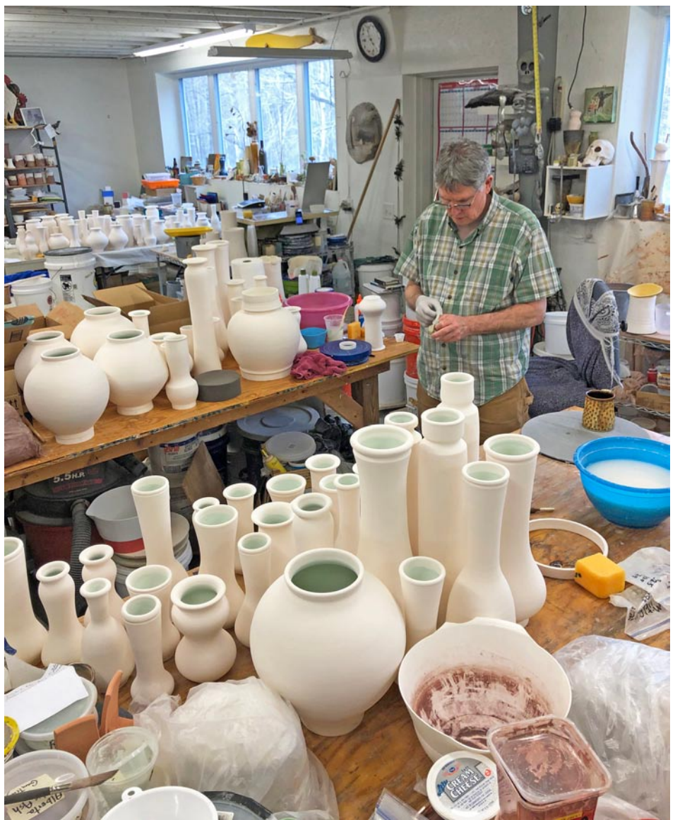
Bruce is fitting rings to the bottom of vases thrown by both him and Samantha Henneke. Hand thrown rings must be custom fitted to each vases' bottom for the crystalline process. Crystalline glaze is very fluid. There will be dish placed under each vase during the firing.
