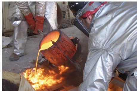
Sand scratch molds filled at iron pour.
